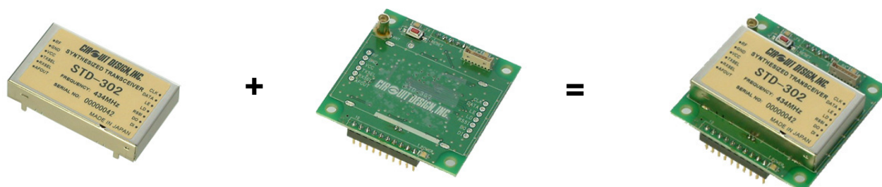
UART interface board (Image shows the UART interface board for STD-302)
