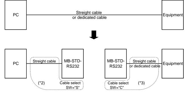
\*2 If cable is cross cable, please set the Cable select SW to "C"
