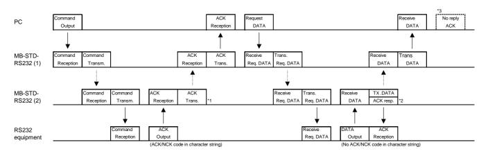
\*1 This is for reply to command from PC. The MB-STD-RS232 does not need to reply with ACK to RS232 equipment
