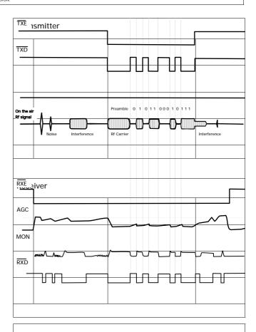
Fig. 4: Transmitter and receiver operation and wave form
